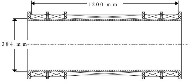
Fig. 3. The geometry of the main magnet
