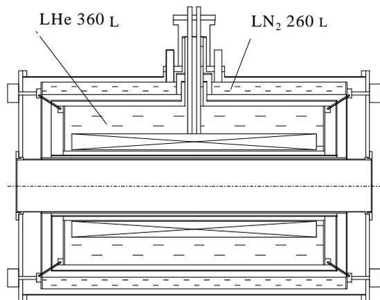
Fig. 6. General layout of the cryostat
