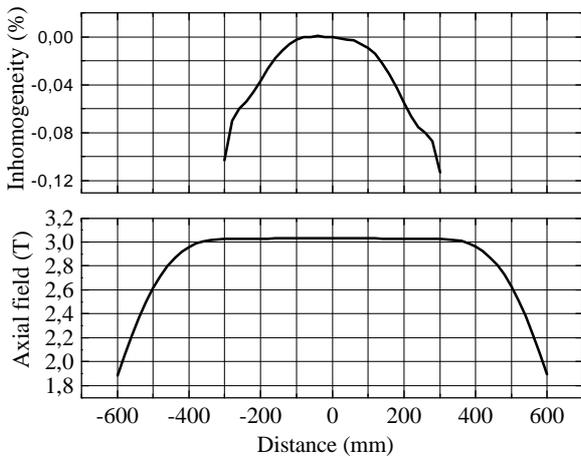
Fig. 4. The field distribution and the homogeneity of the main field along the axis of the magnet.
