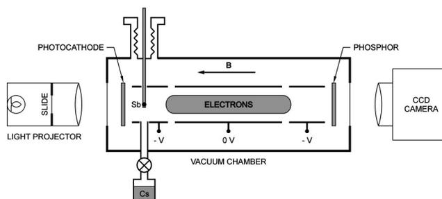
FIG. 1. Geometry of a simple Malmberg-Penning trap with a photocathode electron source and phosphor screen diagnostic. The antimony (Sb) evaporator and cesium (Cs) source are used to fabricate the photocathode.
