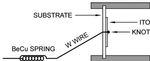
FIG. 7. Simple electric potential control option.
