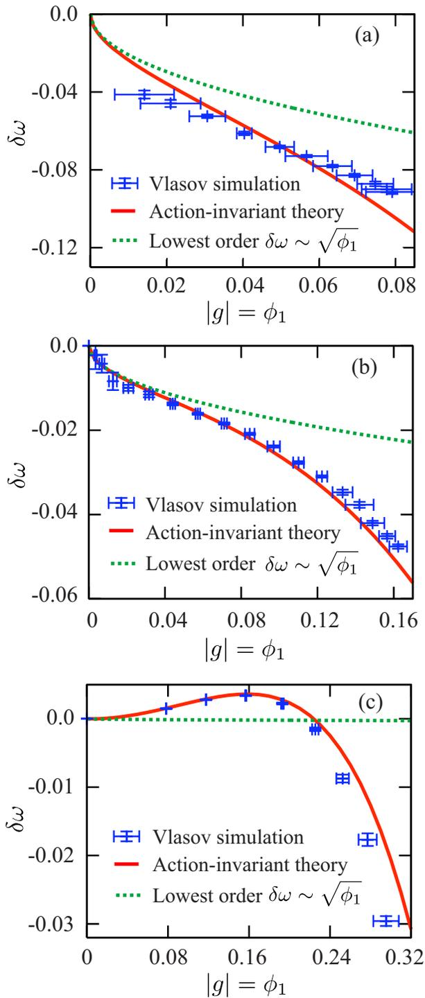
FIG. 1. (Color online) Nonlinear frequency for three different temperatures:  $k_2 \lambda_D = 0.4$  (a),  $0.3$  (b), and  $0.2$  (c). The prediction of the invariant-in-action theory is the solid line, which agrees well with the nonlinear frequency extracted from Vlasov simulations. For comparison, the lowest-order result Eq. (11) is plotted as a dotted line.
